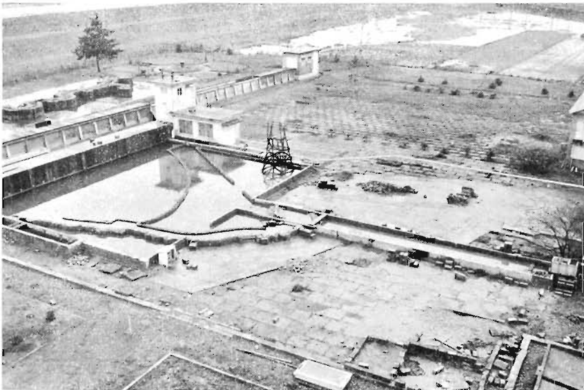
Photo. 10. Model of Sakai Channel for the preliminary experiment.
