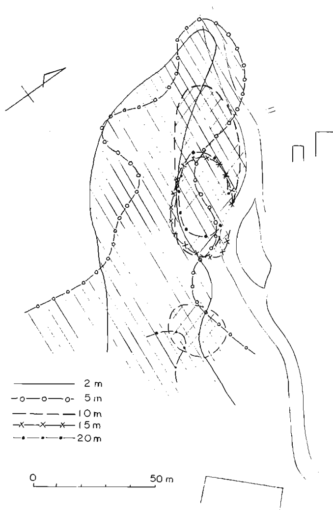
Fig. 8 Horizontal distribution of low apparent resistivity values of 3\text{k}\Omega\text{-cm} or lower ( a=2, 5, 10, 15, 20\text{m} ) on 13th July 1967.
