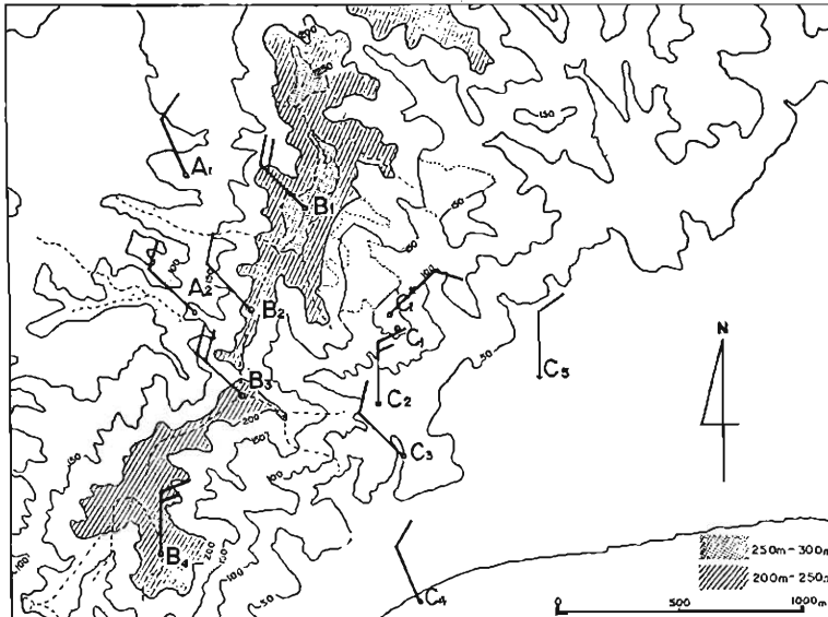
Fig. 3 A typical example of simultaneous wind distribution in the beginning of the reclamation works before the mountain was cut off (mean state from 09 h to 10 h , June 28, 1966). A long blade shows 5 m/sec.
