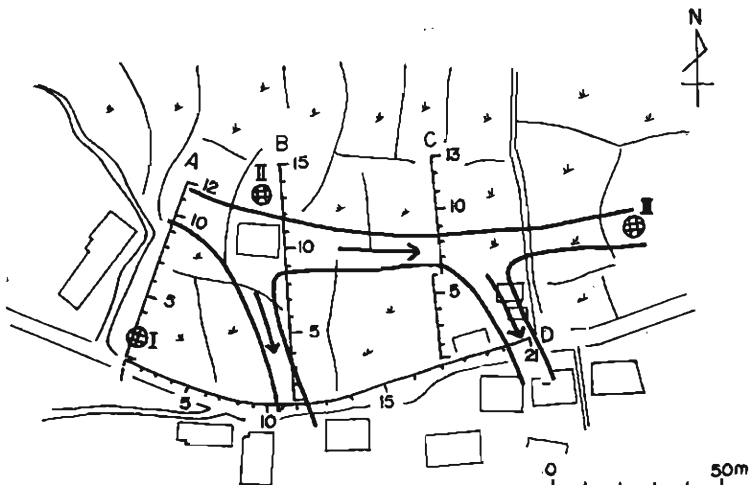
Fig. 6. Measuring lines of underground temperature survey and presumed channel of underground water vein-stream from its result.
