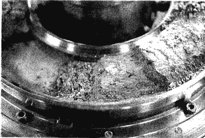
Photo. 4-1. Shear plane of the Shirakawa river sands after the test of Fig. 11-1 . Fine ground sands were observed on the shear plane (at center).
