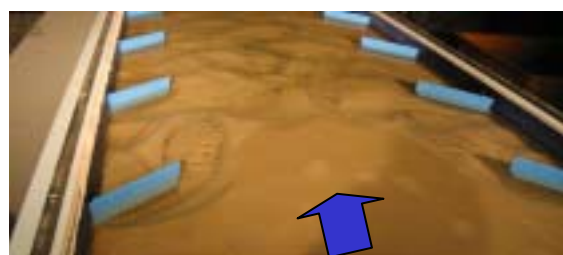
Photo 2. Photograph showing the orientation of bandal plates in a flume test (Rahman, et al., 2004)
