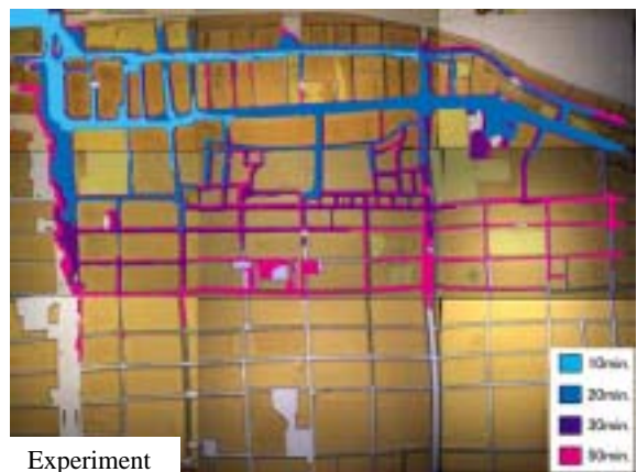
Fig.12 Comparison between flooded area in experiment and that in calculation (intrusion into underground space is not considered)
