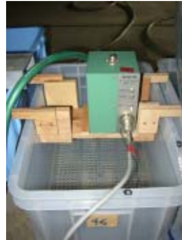
Fig. 5: Servo type water gauge
