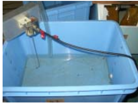
Fig. 4: Capacity type water gauge
