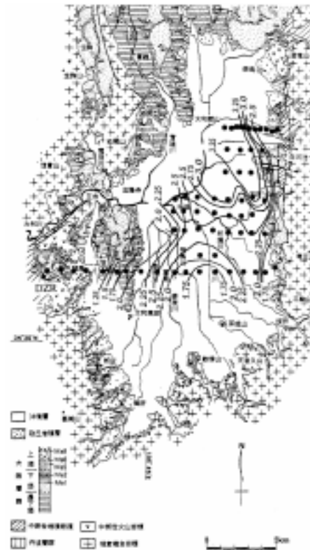
Fig. 8 Peak period of H/V spectral ratio of microseisms. Contour interval = 0.25s. After Morikawa et al.(1998).
