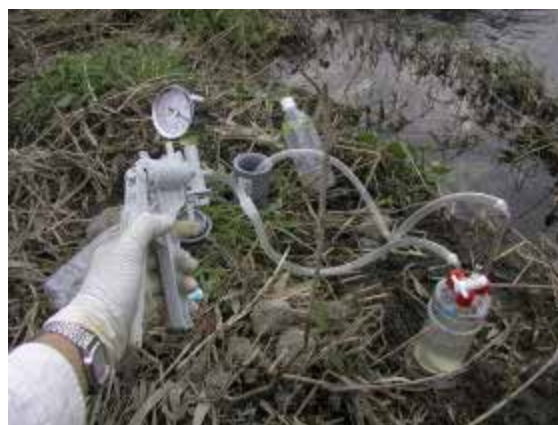
Photo 1 Sampling of river bed inner water
