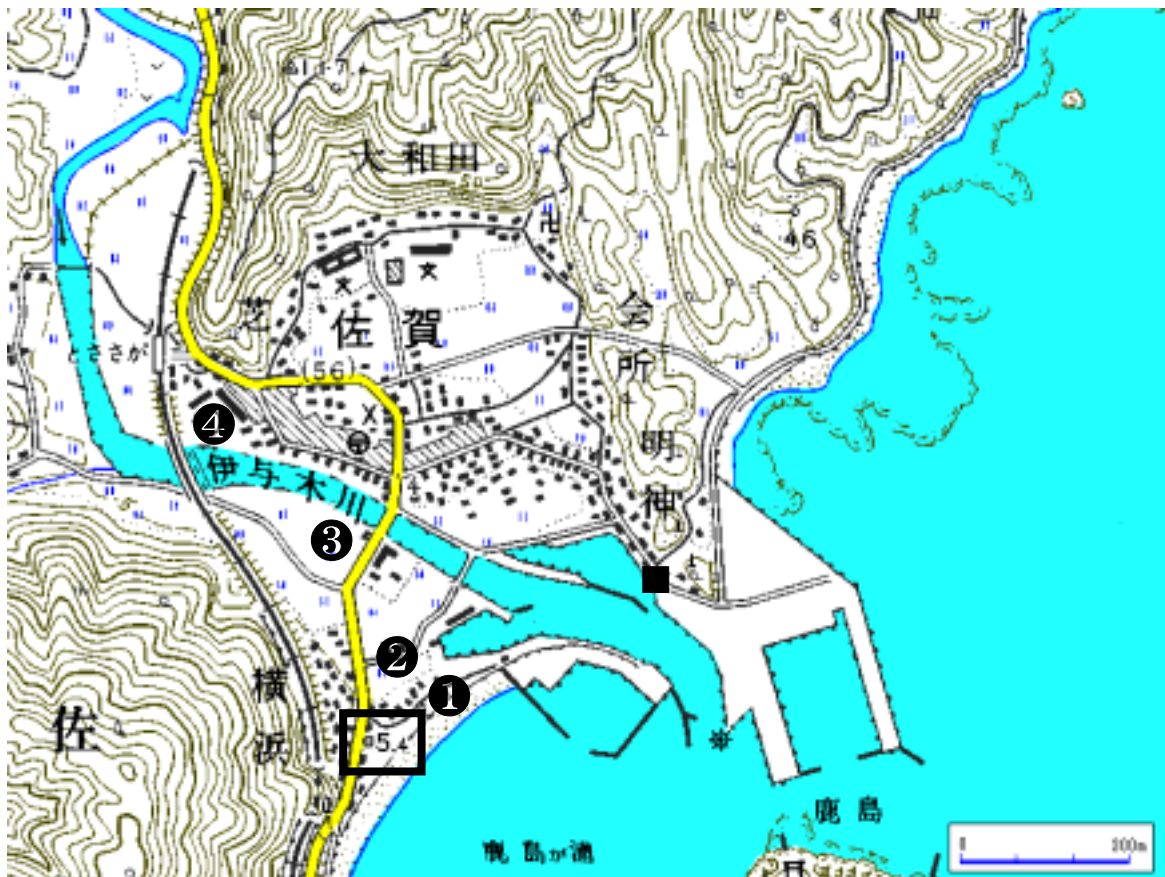
Fig. 2 Layout of the observation stations at Saga. The solid circles No.1, 2, 3, 4 indicate the observation wells. The solid square indicates the tide level observation station. The square indicates the Bench mark.
