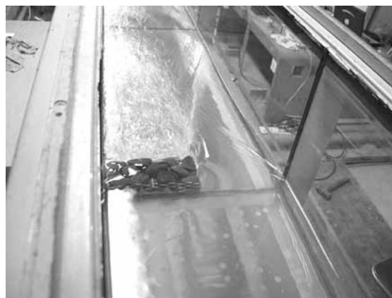
Photo 7 Laboratory experiment on rubble mound groin (Case-B, i.e. h > h_g ).
