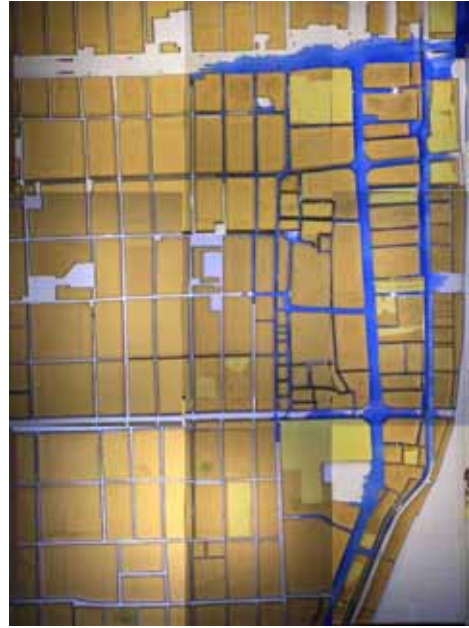
Photo 8 Visualization of inundation. (Case EYD : T=30 min. in prototype)
