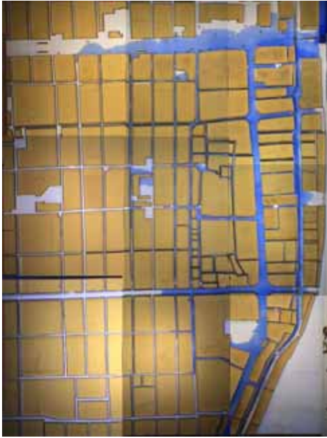
Photo 7 Visualization of inundation. (Case END: T=30 min. in prototype)
