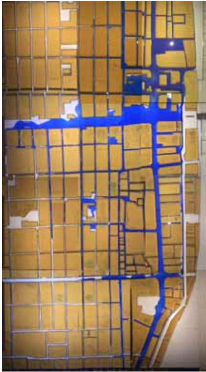
Photo 11 Visualization of inundation. (Case NND: T=30 min. in prototype)
