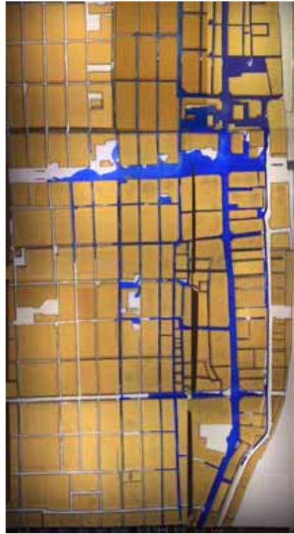
Photo 12 Visualization of inundation. (Case NYD: T=30 min. in prototype)
