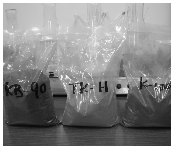
Fig.1: Three types of zero valent iron
