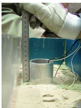
Fig. 11 Uplifted manhole (Case 5)
