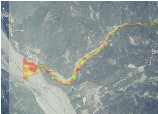
Fig.5 The simulation result – Nantou027, the depth in natural condition case
