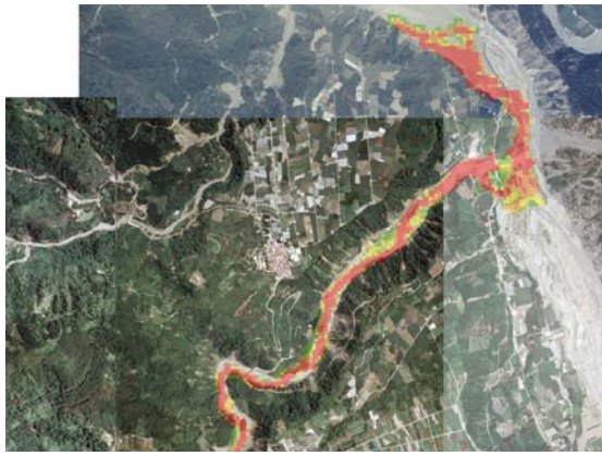
Fig.9 The simulation result – Nantou072, the depth in detention basin condition case
