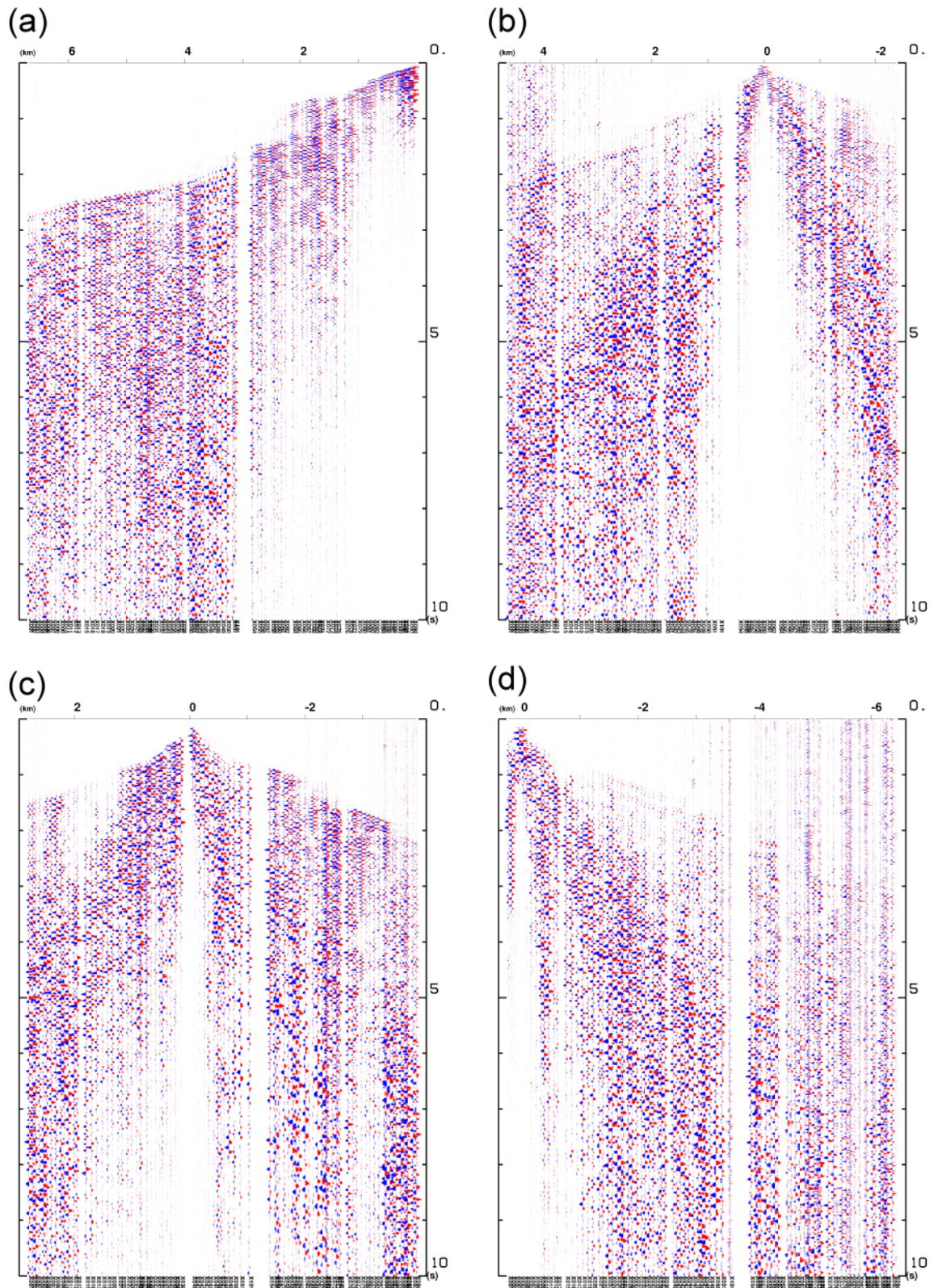
Fig. 5 The 2008 shot record of the linr EW. (a) 08S06, (b)08S11, (c)08S13, (d)08S15. The display style of the panels is the same as that of Fig. 4. After Iguchi et al.(2009).
