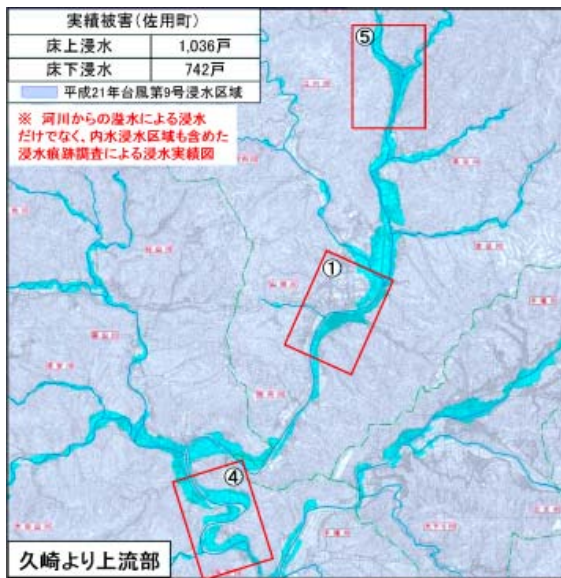
Fig 10 Observed flood inundation area
