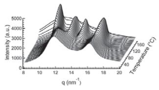
**Figure 1.** WAXD profiles during heating process from 30 to 170  $^{\circ}$ C displayed at every 5  $^{\circ}$ C from bottom to top. The profiles were shifted diagonally for clarification.
