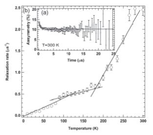
**Figure 2.** (a) Time dependence of the decay of asymmetry for PB at 300 K under a LF of 100 G. (b) Temperature dependence of the decay rate for PB. Lines are shown to clearly observe the onset of relaxation.
