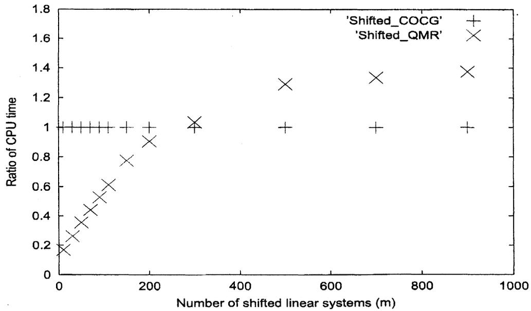
Figure 4: The ratio of the CPU time of the shifted QMR.SYM method to that of the shifted COCG method versus the number of shifted linear systems.
