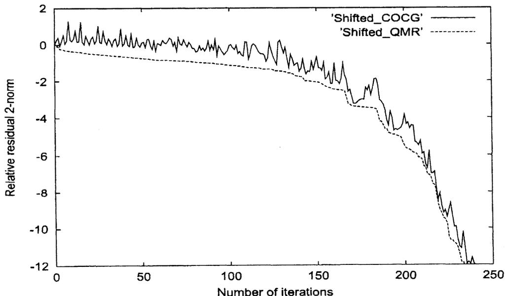
Figure 2:  $\text{Log}_{10}$  of relative residual 2-norms versus the number of iterations of the shifted COCG method and the shifted QMR\_SYM method for shifted linear systems with  $\ell = 701$ , *i.e.*,  $\sigma_{701} = 1.100 + 0.001i$ .
