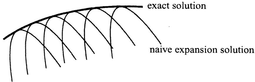
Then, it seems that the envelope gives a good approximate solution. To do this, put  $y = y(\tau)$ , and the envelope is given as follows: At first, we differentiate the family by  $\tau$  at  $t$  and determine  $y(\tau)$  so that the derivative is equal to zero.
