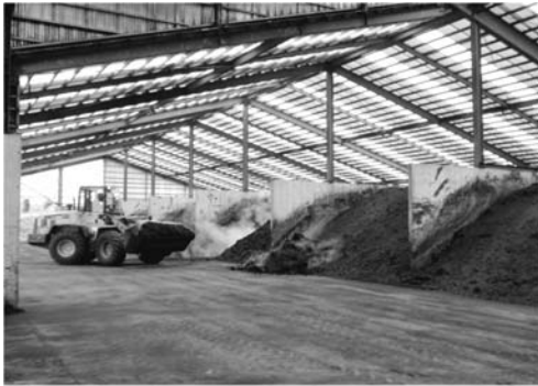
Figure 1. Hyperthermophilic composting of dewatered sewage sludge in aerobic conditions using Bacillus species Source: author
