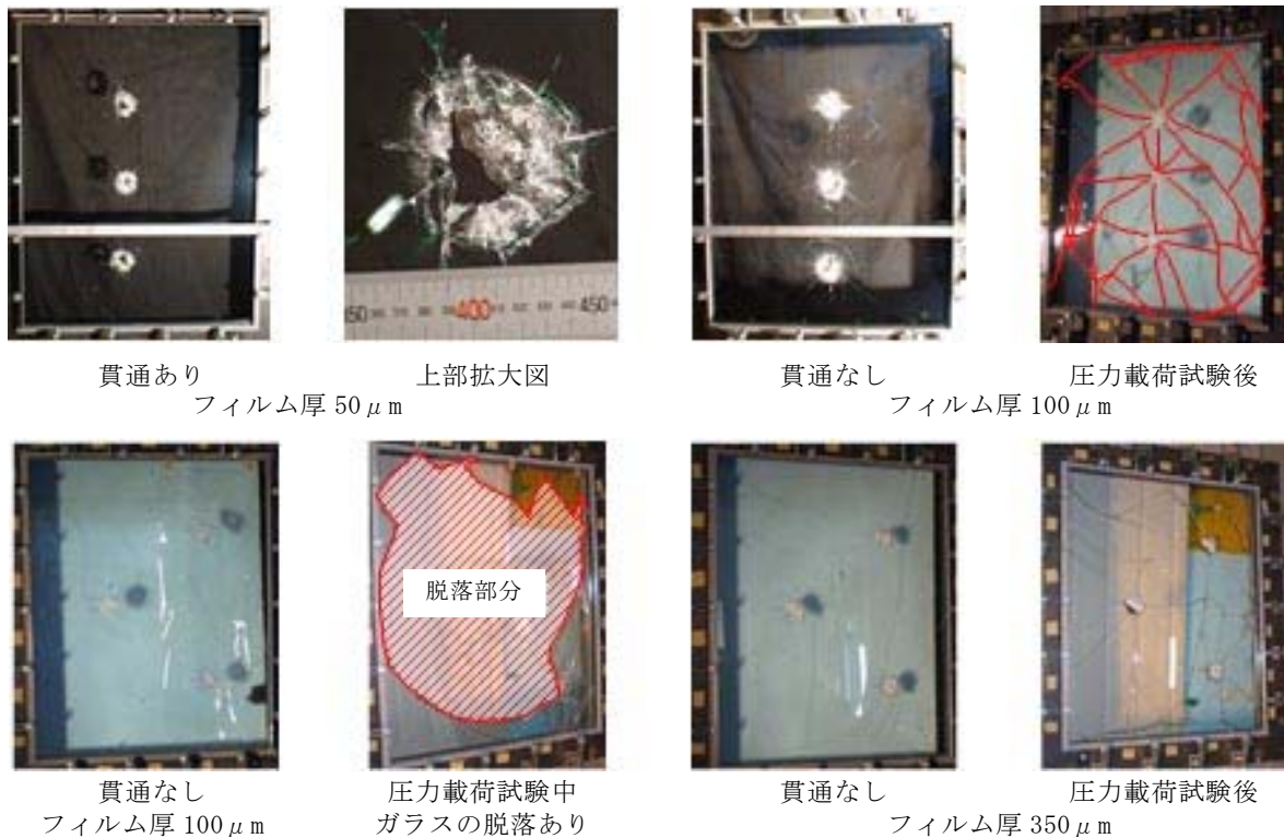
Fig. 18 Results of impact test of partially filmed glasses by missile type A
