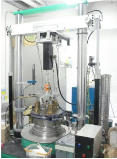
Figure 3: Frontal view of the employed ring shear apparatus DPRI-7
