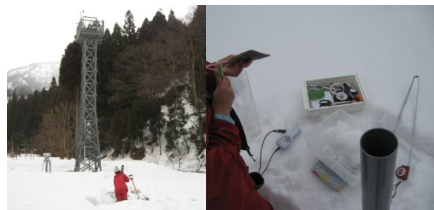
Fig. 2 Surumi station. Right: meteorological equipment and rain gauge. Left: equipment for SWE measurement.
