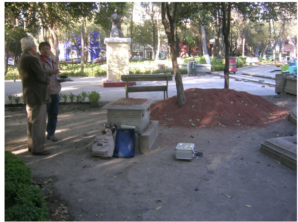
Photo 1 An example of microtremor measurement at one of the strong motion stations of CENAPRED, Jardin Pushkin.
