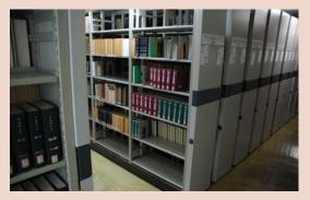
The repair work of the electronic stack as a three-year plan, beginning in 2006 and finishing in March 2009, improved the safety of utilization. One of the upgraded functions is the spread-out function on the passageway of each block. This function allows intervals between shelves, giving them the space which keeps the inside aerated and makes the preserving of books utmost convenient.
