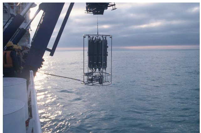
Figure 2. Observation in the Bering Sea during the R/V Mirai MR00-K06 cruise in September 2000.
