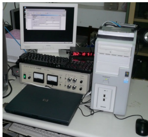
Figure 8. A main amplifier and data recording systems installed inside a room.
