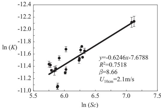
**Figure 3.2** Natural logarithm of K as a function of the natural logarithm of the Schmidt number in the absence of wind-generated capillary ripples (flat interface).
