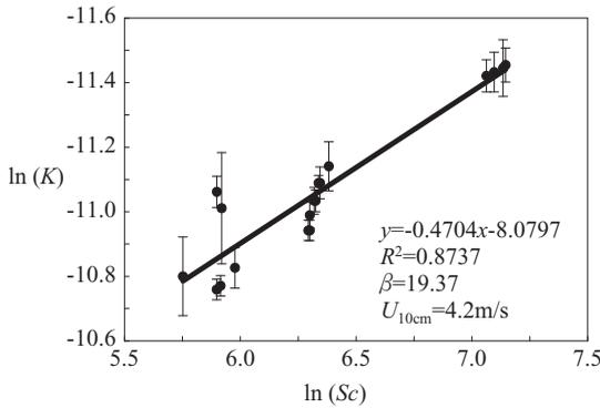
**Figure 3.3** Natural logarithm of K as a function of the natural logarithm of Schmidt number in the presence of capillary ripples.
