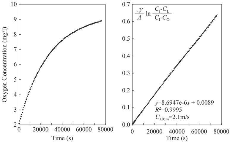
**Figure 3.1** left: Oxygen concentration time series in flat water case at 18°C; right: least-squares fitting for K from equation(4)
