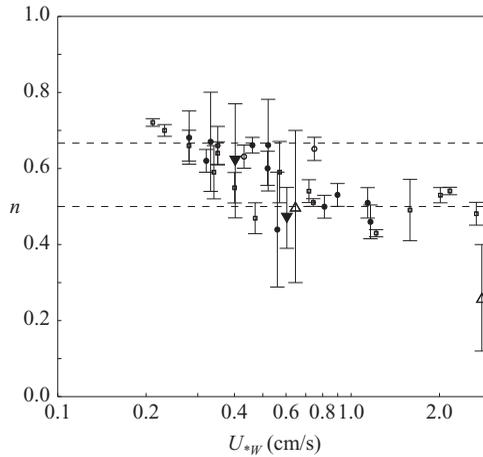
**Figure 3.4**  $n$  as a function of water friction velocity. This figure is modified from Jähne and Haußecker (1998). Open circles, Jähne *et al.* (1998) smooth interface in small facilities; solid circles, Jähne *et al.* (1998) ruffled interface in small facilities; open squares, Jähne *et al.* (1998) ruffled interface in large facilities; open triangles, Wanninkhof *et al.* (1991) in a large linear tank using SF<sub>6</sub> and N<sub>2</sub>O; downward pointing solid triangles, this study.
