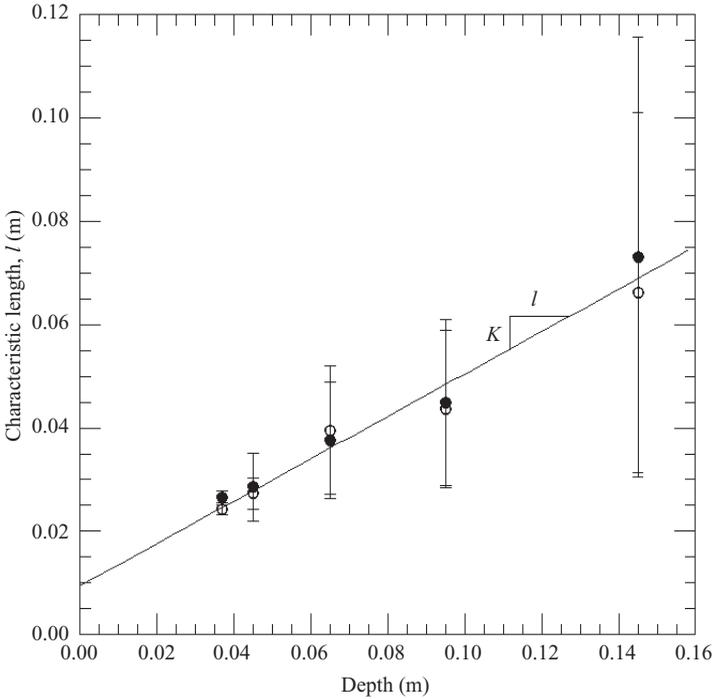
**Figure 6** Vertical profile of the turbulent integral length scale ( $l$ ) obtained from the intensity spectra (ADV mounted on a moving trolley measurements). The dashed line shows a linear fit with a slope equivalent to the Von Karman parameter,  $\kappa=0.41$ .
