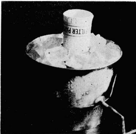
Fig. 3. Refrigerator (made of stainless steel) for anaesthetizing insects.
