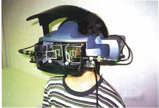
▲写真1. 視覚系情報収集機能付き HMD (Eye-sensing Head Mount Display)
