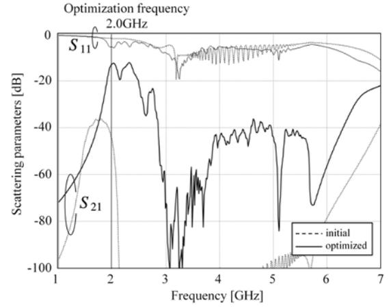
Fig 3. Frequency characteristics of scattering parameters  $S_{11}$  and  $S_{21}$  of Example 1, maximizing  $S_{21}$  at 2.0 GHz
