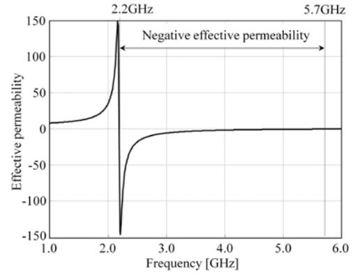
Fig 8. Effective permeability curve of the ferrite material.
