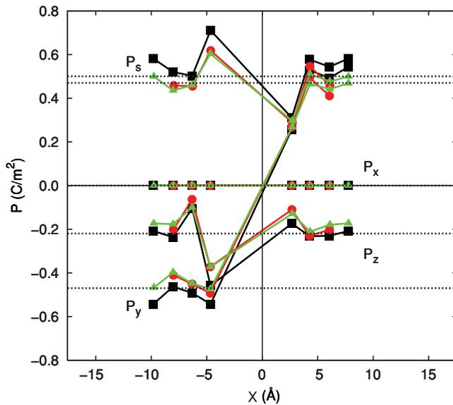
FIG. 8. (Color online) Comparison of the polarization profiles evaluated using DFT in the vicinity of the  $\Sigma 5(201)$  GB for supercells with 16 formula units (dots, red) and 20 formula units (triangles, green), and using SMP with 20 formula units (squares, black). Results obtained with both SMP and DFT show good agreement.
