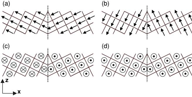
FIG. 1. Schematic sketch of the  $\Sigma 5(201)$  grain boundaries with different polarization arrangements in adjacent grains (domains) for supercells with 20 unit cells. (a)  $127^\circ$  DW; (b)  $53^\circ$  DW; (c)  $180^\circ$  DW; (d)  $0^\circ$  polarization change (without a DW). Microscopic translations of grains with respect to each other are disregarded here.
