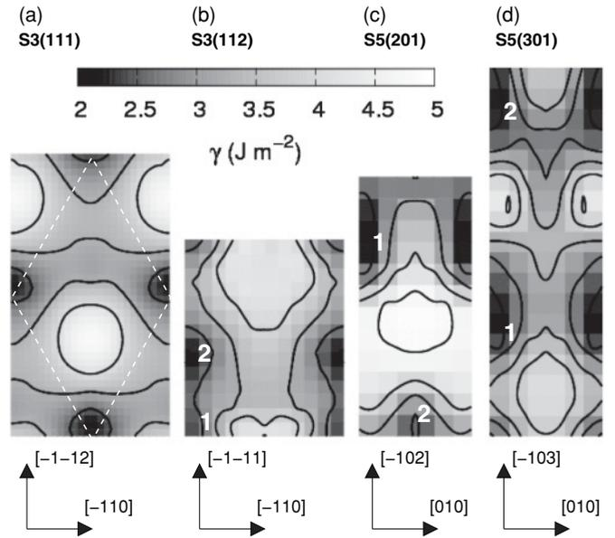
FIG. 3.  $\gamma$  surfaces as obtained from the atomistic SMP simulations. For  $\Sigma 5$  GB the  $(201)^{53^\circ}$  and  $(301)^{37^\circ}$  variants are displayed. Lighter gray indicates a higher energy, and darker gray indicates a lower energy (the grayscale is the same for all four plots). Nonequivalent local minima in the energy are referred to in the text by the displayed numbers. The broken lines in  $\Sigma 3(111)$  indicate the  $y$ - $z$  cross-section area of the used supercell.
