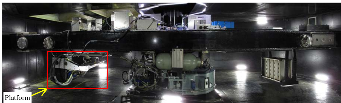
Photo 1 Side view of new geotechnical centrifuge at DPRI
