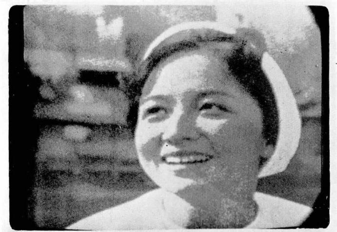
(a)  $f_s = 10 \text{ Mc}$ ,  $f_w \approx 3.5 \text{ Mc}$ , 4レベル量子化
