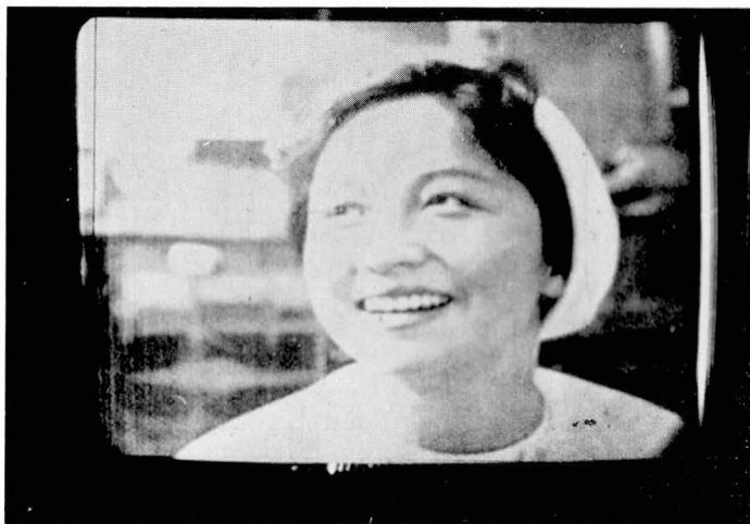
(b)  $f_s = 20 \text{ Mc}$ ,  $f_w \approx 7 \text{ Mc}$ , 2レベル量子化
