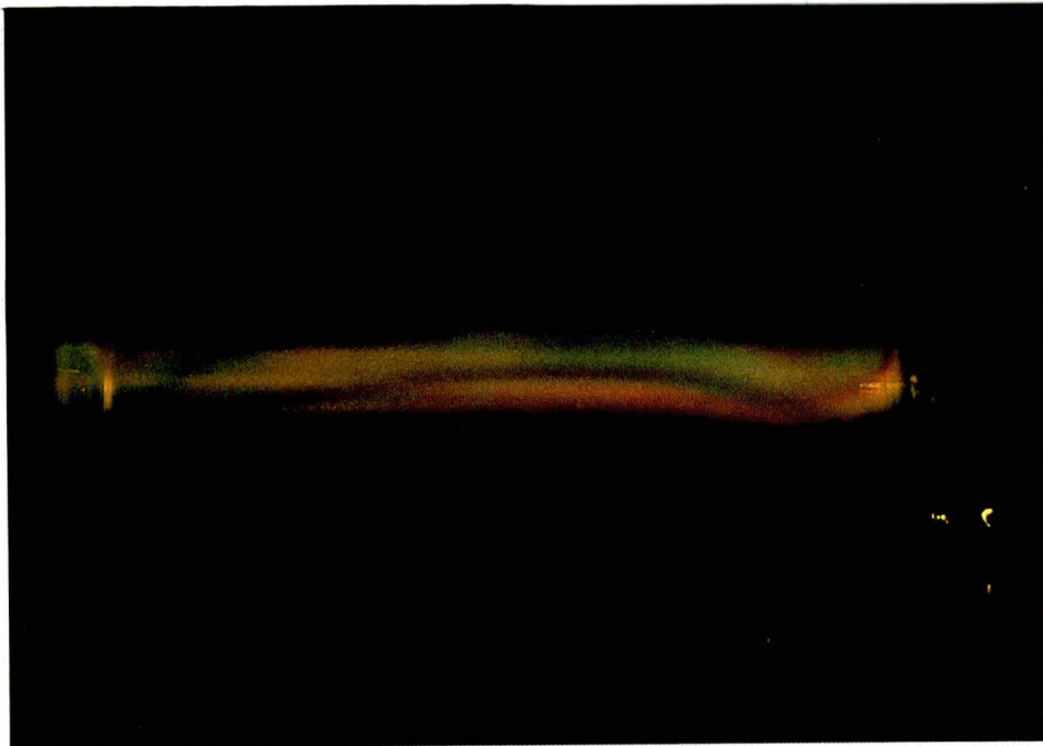
Fig. 3.20 A photograph of the white light scattering by CsH laser snow produced by the \text{Ar}^+ laser 457.9 nm line. The white light beam diameter was about 10 mm and the \text{Ar}^+ laser beam diameter was about 15 mm. The cell temperature was 334^\circ\text{C} and the \text{Ar}^+ laser power was 210 mW. In this figure, we can see both the stripes of the scattered light intensity and the changes of color or wavelength. This means that there are spatial distributions of both the particle density and the particle size. (See pages 75 and 134.)
