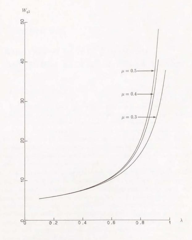
Figure 3.7: Average waiting time in queue 1 for K = 3,  $\alpha = 0.2$ ,  $\gamma = 0.2$ .
