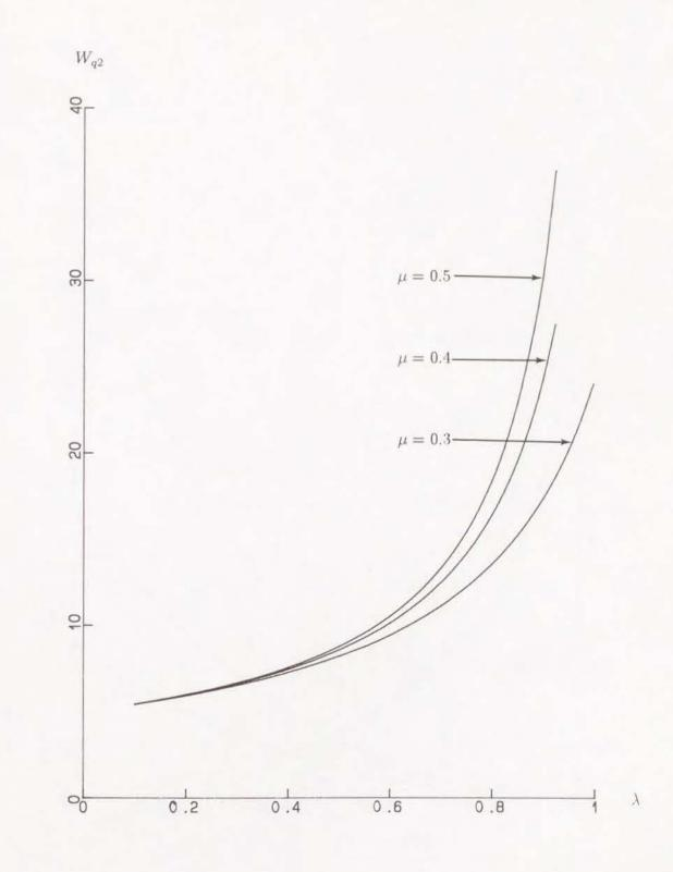
Figure 3.4: Average waiting time in queue 2 for K = 2,  $\alpha = 0.2$ ,  $\gamma = 0.2$ .
