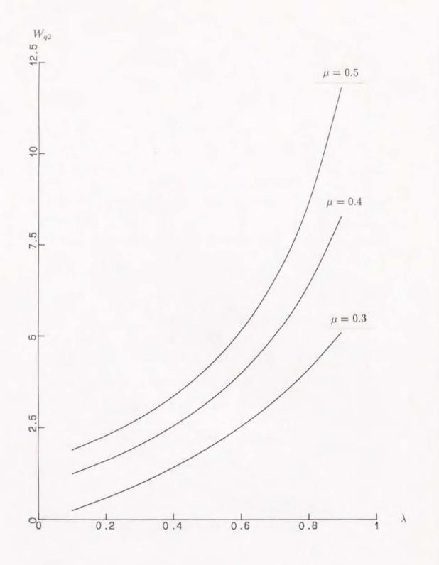
Figure 2.3: Average waiting time in queue 2 for  $\alpha = 0.2$ ,  $\gamma = 0.2$ .
