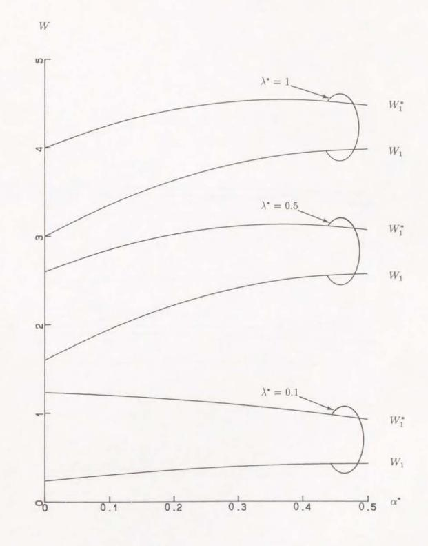
Figure 4.2: Average ordinary and set-up waiting time for  $\mu_1 = \mu_2 = 0.5$ ,  $\nu_{12} = \nu_{21} = 0.5$ .
