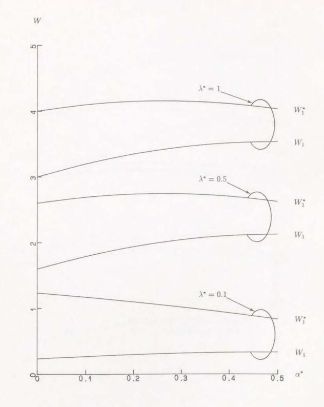
Figure 4.6: Average ordinary and set-up waiting time for  $\mu_1 = \mu_2 = 0.5$ ,  $\nu_{12} = 0.1$ ,  $\nu_{21} = 0.5$ .
