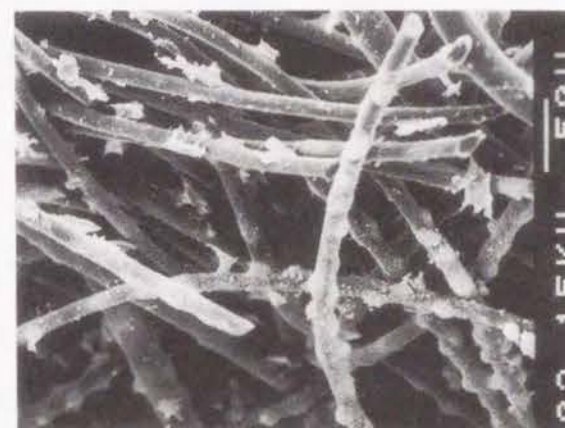
Figure 4.4. Scanning electron microphotograph of the cultured chondrocytes attached to the PLLA scaffold.
