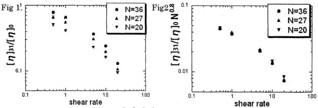
We have found that the ratio  $[\eta]_{\mathbb{K}}/[\eta]_{31}$  is expressed as a quadratic function of ACN(N) and shear rate  $\gamma$ . In the case of high shear rate, we have
