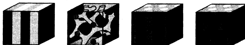
Figure 1: Morphology of AB block copolymer systems. Light and dark gray correspond to A and B components of AB block copolymers, respectively. With decreasing the fraction of the A component, the shape of A component becomes lamellae, bicontinuous double gyroid struts, cylinders, and spheres. The lattice constants (periodic lengths) are the order of 10-100 nm.
