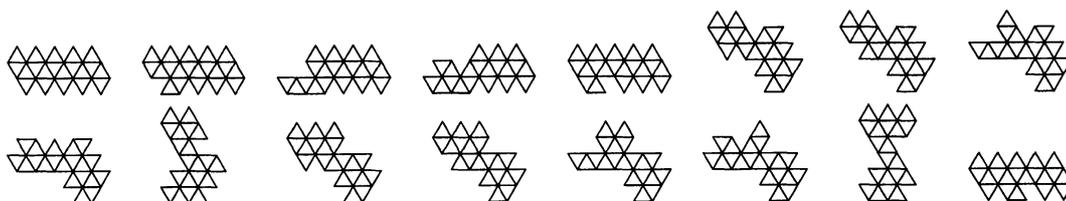
Figure 2: Partial List of Edge-Developments of an Icosahedron.
