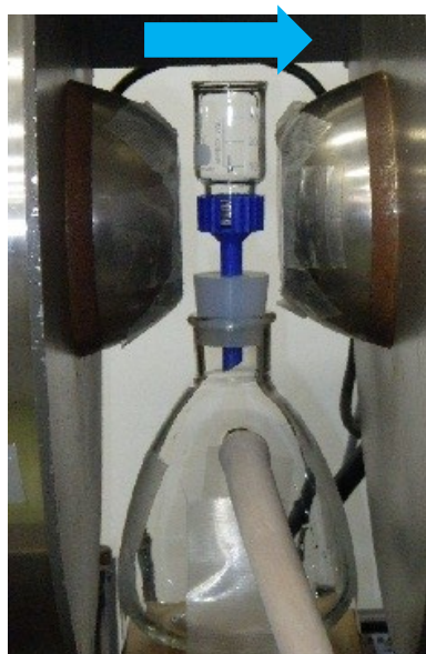
Fig.1 Apparatus for filtration under reduced pressure with application of a static magnetic field. An arrow indicates direction of a magnetic field.
