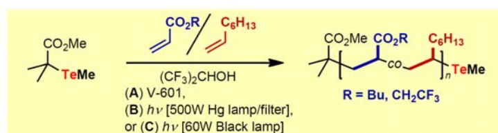
Scheme 6. Copolymerization of acrylate and 1-octene under TERP
