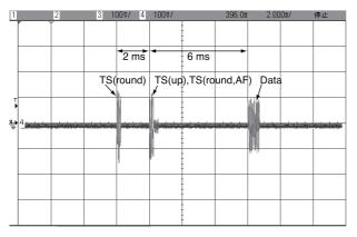
Fig. 7 Timing of packets observed using the oscilloscope.
