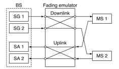
**Fig.8** Experimental setup for in-lab experiments. SGs and SAs of the BS equipment are directly connected with the fading emulator.
