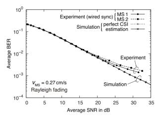
Fig.9 BER versus SNR performance over the slow Rayleigh fading channel ( $v_{MS} = 0.27$  c/ms).
