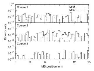
Fig. 14 BER performance for the three MS courses. BER is calculated every  $30 \text{ cm} \simeq 5\lambda$ .
