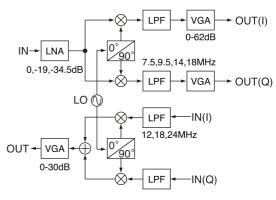
Fig. 5 Block diagram of the transceiver chip.
