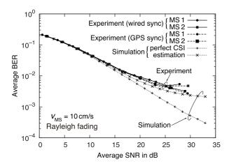
Fig. 10 BER versus SNR performance over the faster Rayleigh fading channel ( $v_{MS} = 10$  c/ms).
