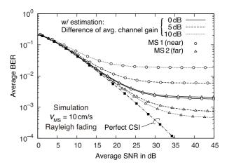
Fig. 17 SNR versus BER performance with channels from/to MS 2 attenuated by 0, 5, 10 dB.
