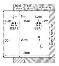
Fig. 12 Layout of the experimental location.
