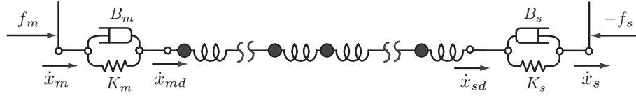
Fig. 4.2 Physical interpretation of symmetric-type wave-variable-based teleoperator.
