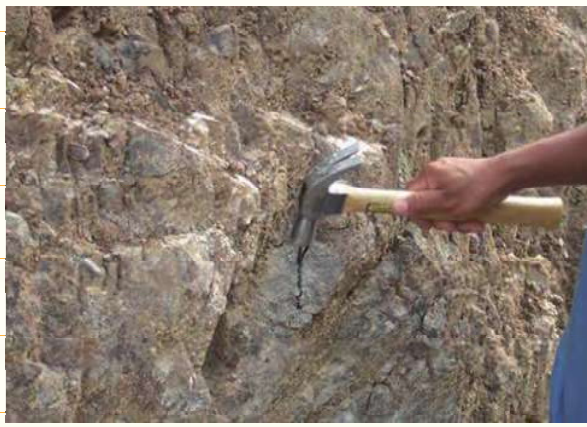
Figure 11-2: Sample photos of very blocky and fractured soft rock [source: DRH 61]
