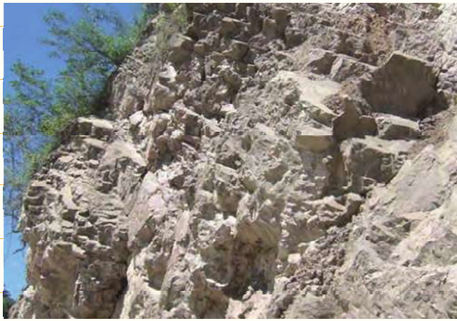
Figure 8-2: Samples of very blocky, fractured and disturbed hard rock [source: DRH 61]
