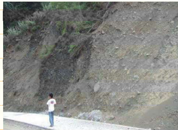
Figure 12-2: Sample photos of stiff, cemented and dense gravelly, sandy, silty and clayey soils [source: DRH 61]
