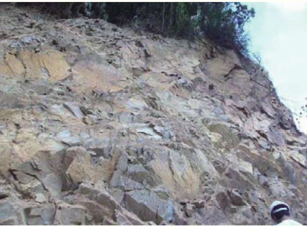
Figure 8-2: Samples of very blocky, fractured and disturbed hard rock [source: DRH 61]
