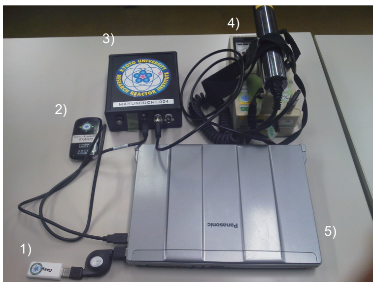
Figure 2: The in-vehicle part is compactly composed of mostly commercial components. 1) GPS unit, 2) 3G mobile wi-fi router, 3) MAKUNOUCHI, 4) NaI survey meter, 5) PC.
