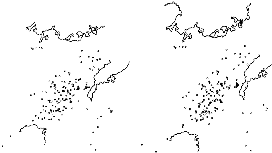
Fig. 1a. Distribution of epicenters of the micro-earthquakes for the assumed velocity of 5.5 km/sec.
